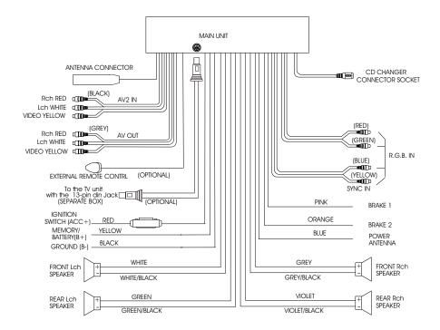
**Note:** The Brake 1 wire is designed to connect to the ground wire, and the Brake 2 wire is designed to connect to CPU. Be sure that these two wires can't be connected to other wires, especially the ACC+ wire and the B+ wire.
